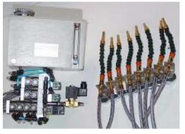
eight micropumps in three groups a solenoid valve two manual valves a five litre tank with a low level switch eight stainless steel sheathed coaxial hoses eight flexible coaxial nozzles with fixing magnets.
